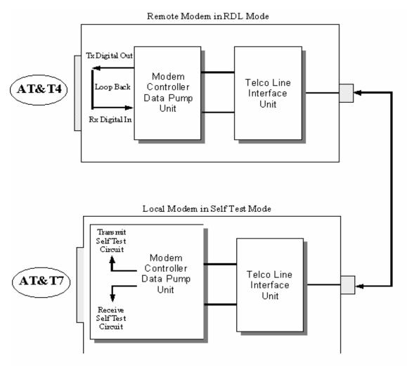
Figure 5 REMOTE DIGITAL LOOPBACK WITH LOCAL SELF TEST
